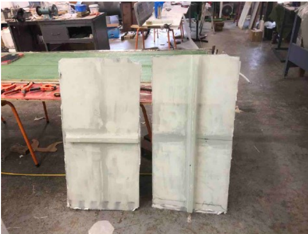
Coreless bulkheads. Bit more work and a little heavier than say 600 gsm either side of 20mm foam, but a lot stiffer and cheaper. The next ones will have half the laminate, and flanges on all sides for easy fitting in the lee hull.
