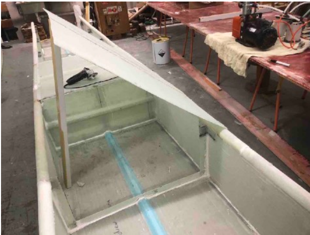
Toy box hinges: The edge stiffening tubes are used as hinge pins for the toy box covers.
