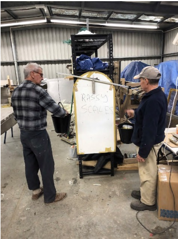
Rassy scale and balance weight. Simple and near idiot proof. One less thing to worry about during an infusion. Thanks Rob R.
