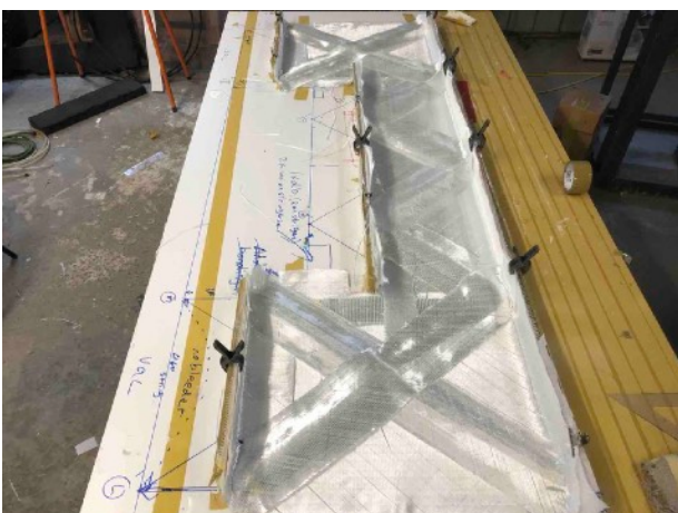
No foam bulkhead ready for plumbing
