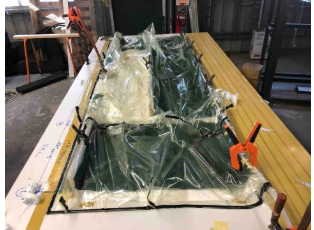
No foam bulkhead ready to infuse
