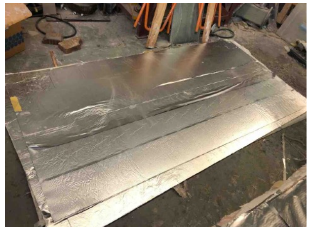
Wing leading edges with alu foil
