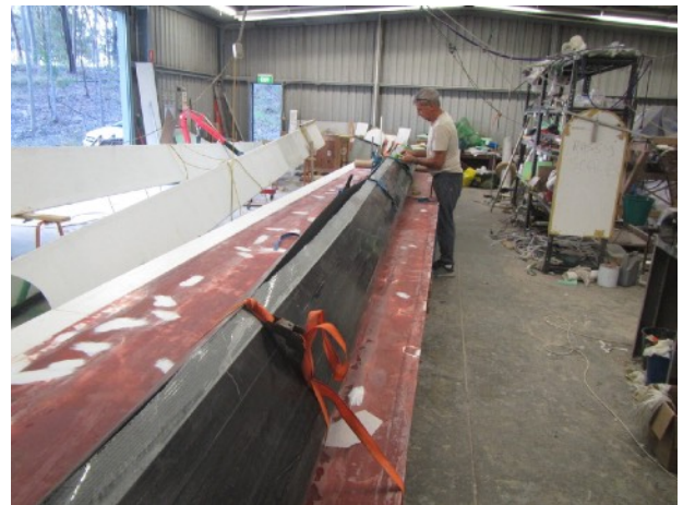
Joining mast mid section
