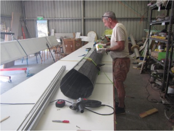
Joining mast top
