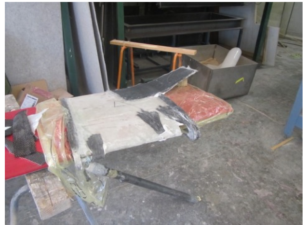
Rudder case addition
