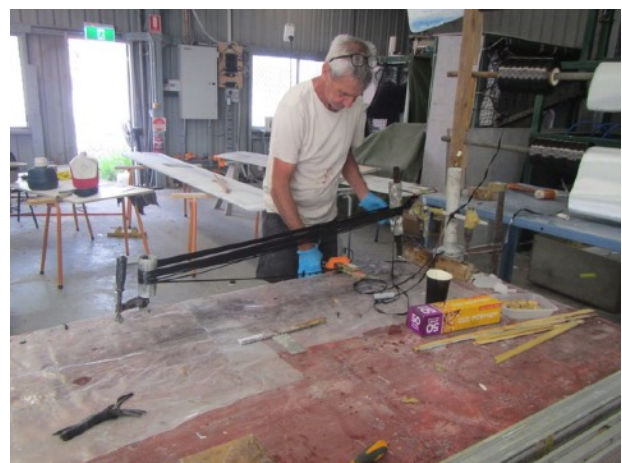
Building wing battens
